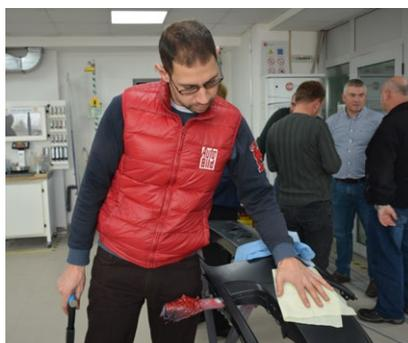
When the surface of the car body is polished, electrical charge develops
