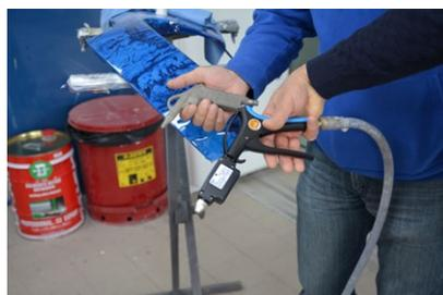
The mechanism is embodied in the "head" of the IONSTAR. It consists of a tiny turbine and a dynamo which is driven by the airstream from the compressed air. Other than that, IONSTAR resembles any other conventional compressed air gun
